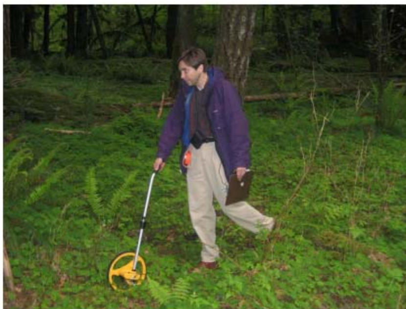
Figure 3-10. Measuring course length with measuring wheel.
