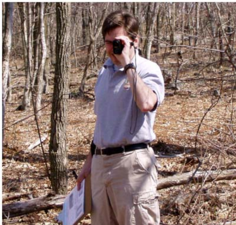
Figure 3-8. Hand-held Laser Range Finder in use.
