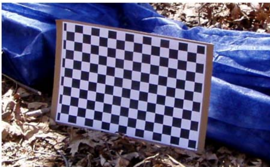
Figure 3-6. Vegetation Density Board.
