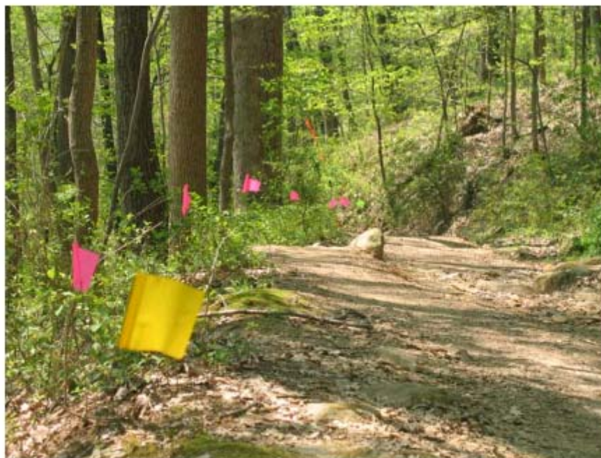
Figure 3-9. Track marked with several different colors of surveyor's flags. Yellow flags used for start, every 500 meters, and finish. Green flag marked with distance every 25 meters, red flags help clearly mark the track. Flagging tape used to initially layout the track.
